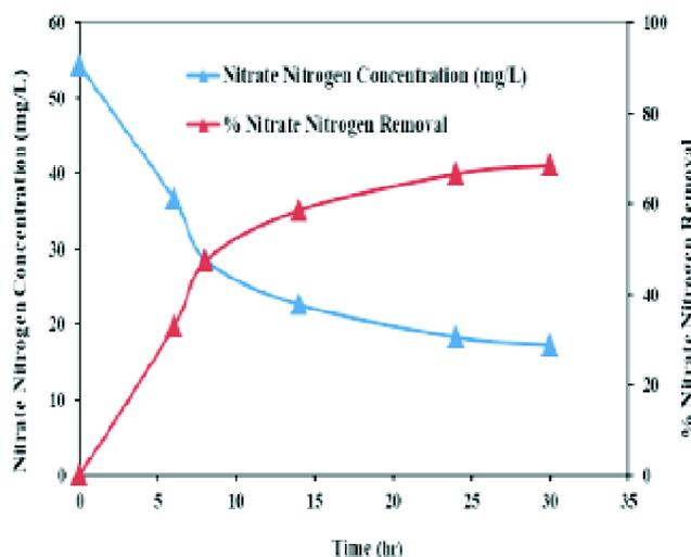
Fig. 5. Nitrate nitrogen removal profile in batch reactor [initial  $\text{NO}_3^-\text{-N}$  = 54.36 mg/L].
