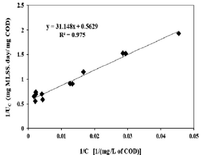
Fig. 8. Graphical plot for substrate utilization kinetics for carbon oxidation.
