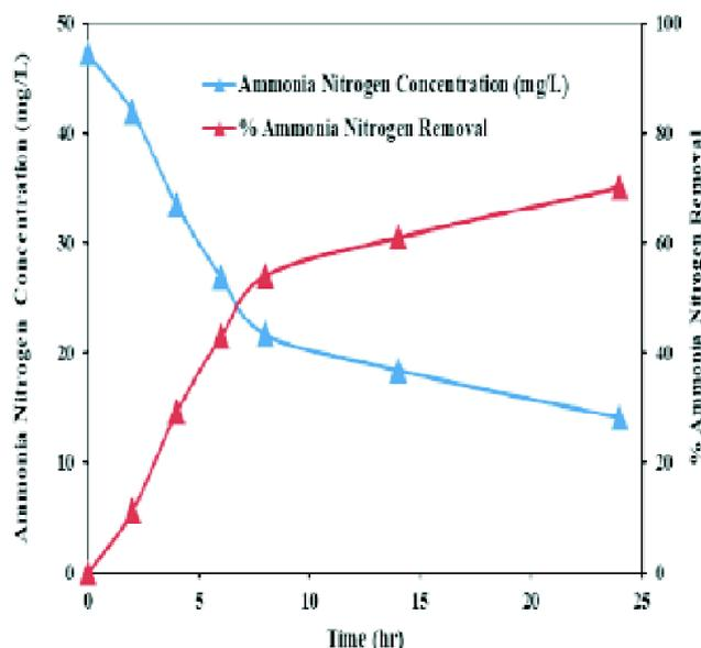
Fig. 4. Ammonia nitrogen removal profile in batch reactor [initial  $\text{NH}_4^+\text{-N}$  = 47.2 mg/L].
