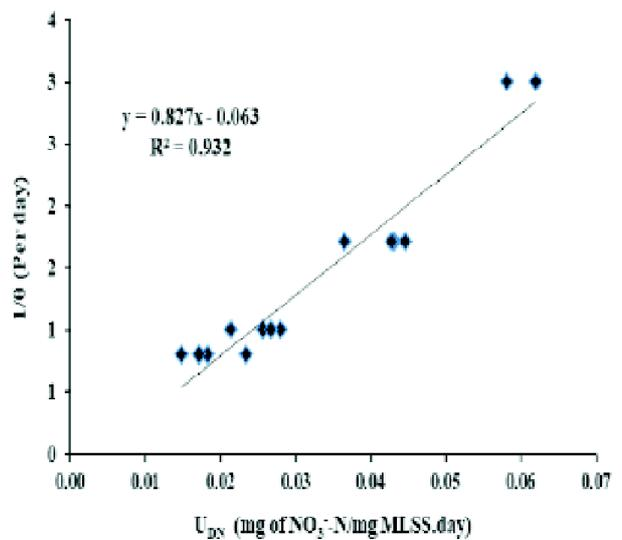
Fig. 13. Graphical plot for microbial growth kinetics for denitrification.
