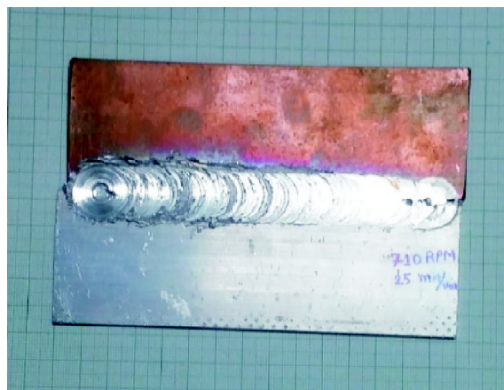
Fig. 3. FSW Joint (AA 6061-T6 and Cu B370).
