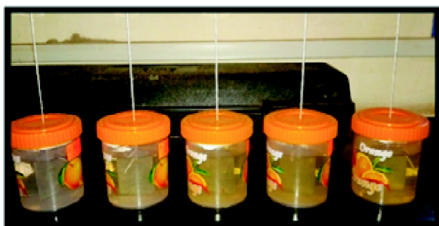
Fig. 1. Experimental set up for the Hibiscus leaf extracts as corrosion inhibitor.
