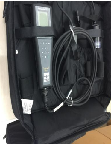
Fig. 1. YSI ProQuatro Multi Parameter for Measuring Temperature, Dissolved Oxygen, Salinity, and pH.
