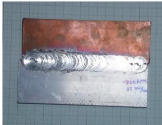
Fig. 3. FSW Joint (AA 6061-T6 and Cu B370)
