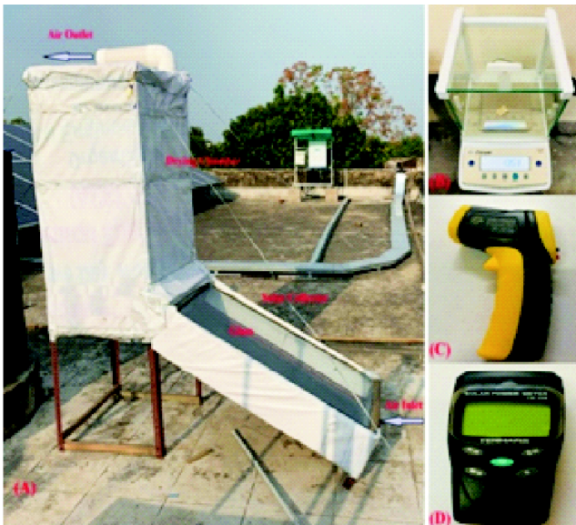
Fig. 1. (A) Indirect type solar dryer experimental setup, (B) weighing machine, (C) infrared thermometer and (D) solar power meter.
