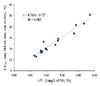
Fig. 12. Graphical plot for substrate utilization kinetics for denitrification.
