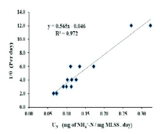
Fig. 11. Graphical plot for microbial growth kinetics for nitrification.
