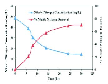
Fig. 6. Nitrate nitrogen removal profile in batch reactor [initial NO<sub>3</sub><sup>-</sup>-N = 48.67 mg/L].
