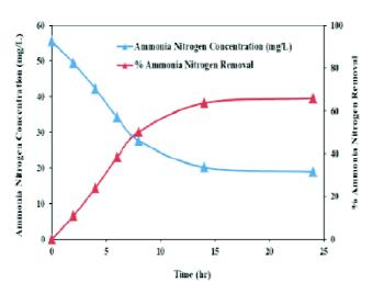
Fig. 3. Ammonia nitrogen removal profile in batch reactor [initial NH<sub>4</sub><sup>+</sup>-N = 55.4 mg/L].
