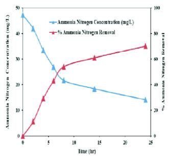
Fig. 4. Ammonia nitrogen removal profile in batch reactor [initial NH<sub>4</sub><sup>+</sup>-N = 47.2 mg/L].
