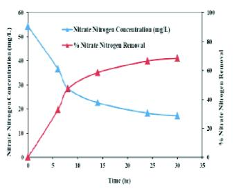
Fig. 5. Nitrate nitrogen removal profile in batch reactor [initial NO<sub>3</sub><sup>-</sup>-N = 54.36 mg/L].
