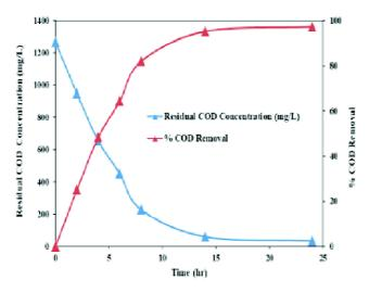
Fig. 2. Carbon oxidation profile in batch reactor [initial COD = 1266 mg/L].
