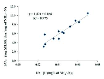
Fig. 10. Graphical plot for substrate utilization kinetics for nitrification.
