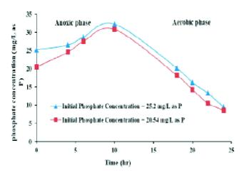
Fig. 7. Phosphorous removal profile in batch reactor.
