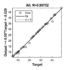
Fig.1. Regression plot of experimental versus predicted values for the optimum ANN model.
