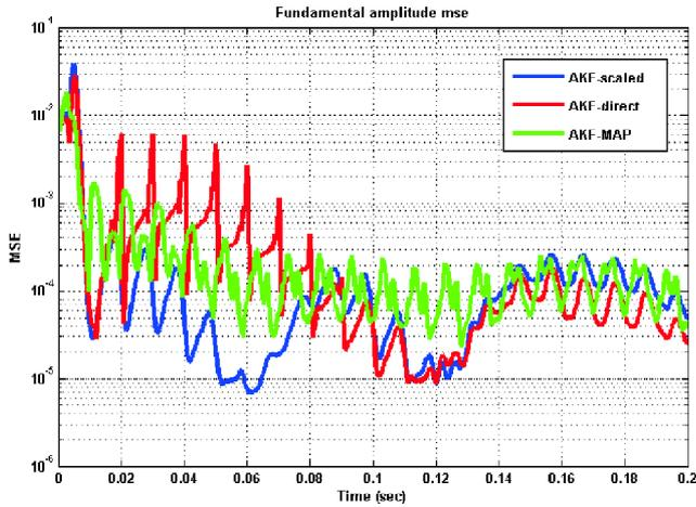
Fig. 6. Fundamental amplitude MSE and error covariance for 500 MC runs.
