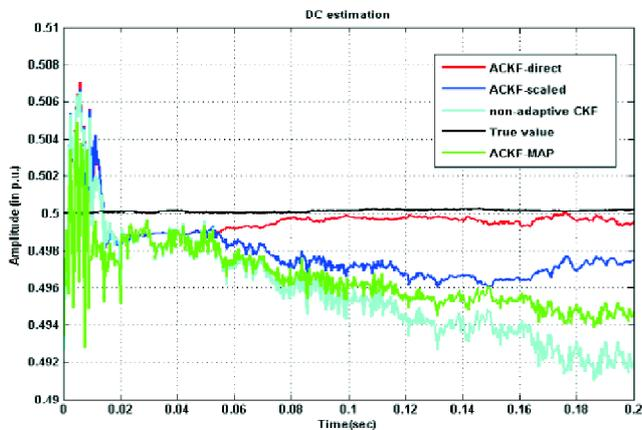
Fig. 7. True and estimated DC amplitude for representative run.
