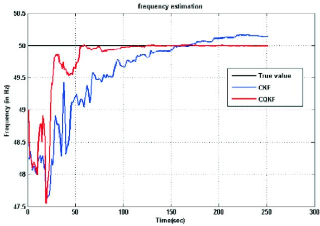
Fig. 10. True and estimated fundamental frequency for a representative run.
