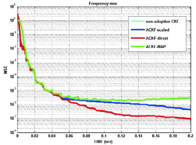
Fig. 8. Frequency MSE for 500 MC runs.
