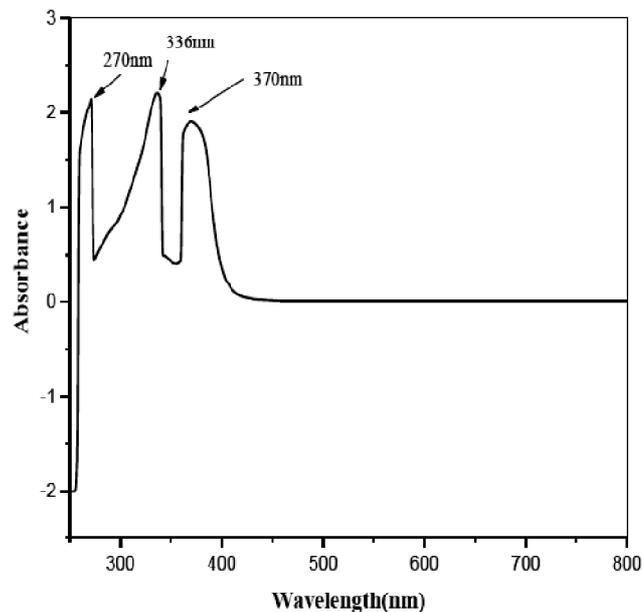
Fig. 5. UV-Visible spectrum of DMBDPP.
