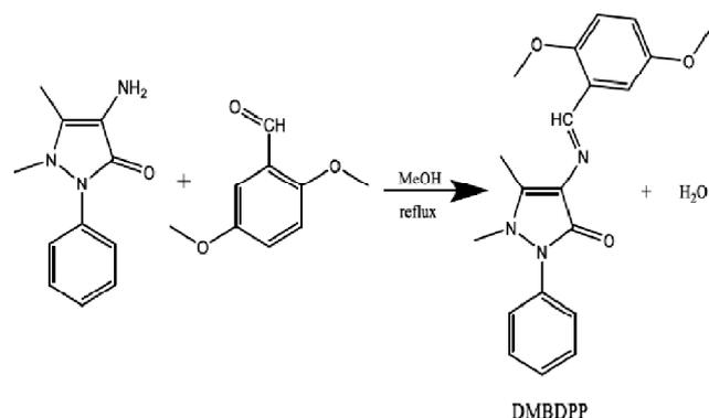
**Scheme 1.** Synthesis of 4-(N-2,5-dimethoxybenzaldehyde)-2,3-dimethyl-1-phenyl-3-pyrazolin-5-one (DMBDPP).
