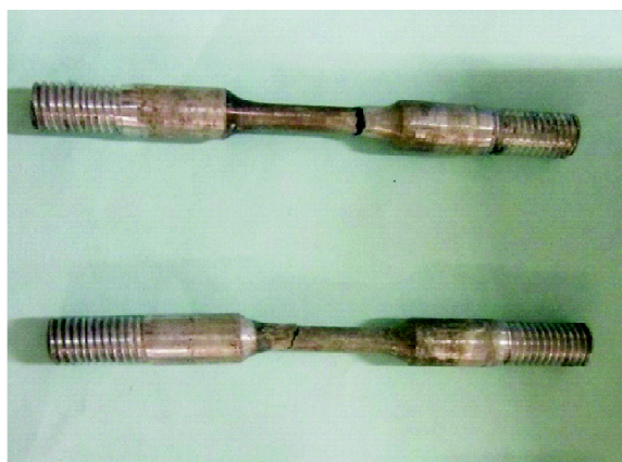
Fig. 2. Sulphide stress corrosion cracking tested samples.
