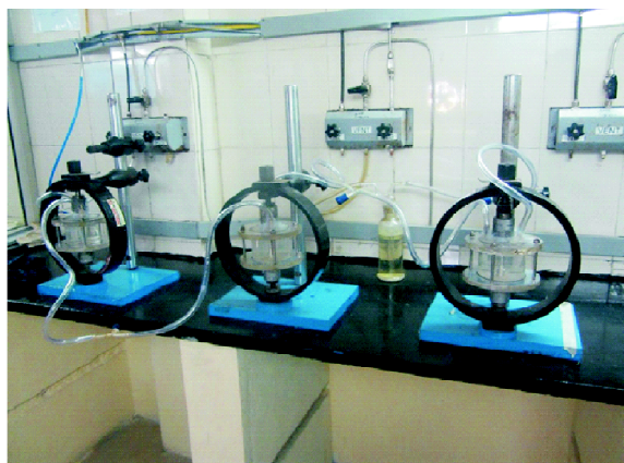
Fig. 1. Photograph of sulphide stress corrosion cracking apparatus.
