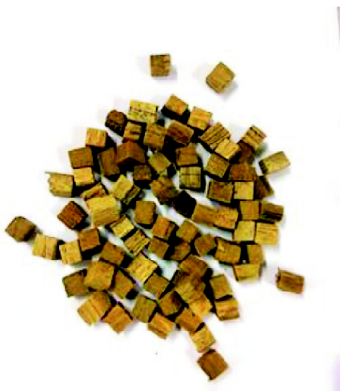
Fig. 2. Low density wood particle used as biocarrier.
