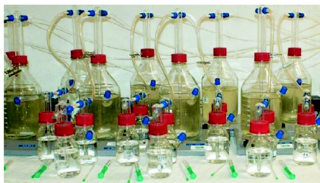
Fig. 7. Pictorial view of sturm test biodegradation being performed in laboratory.
