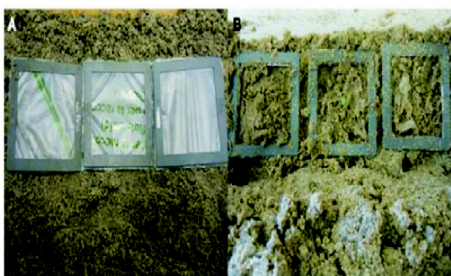
Fig. 5. Picture showing soil burial treatment in a domestic garden.
