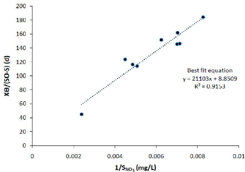
Fig. 4. Determination of  $K_s$  and  $k$ .
