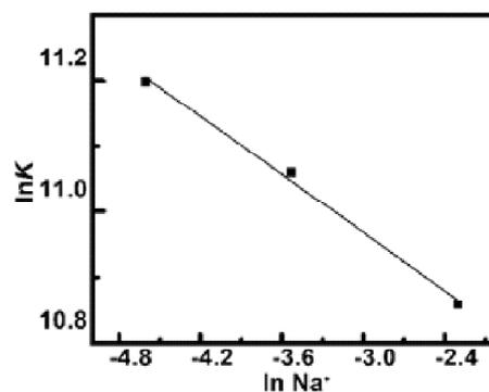
Fig. 5. Van't Hoff plot for Hb-SMZ binding from salt dependent fluorescence quenching at 10, 30 and 100 mM concentrations.
