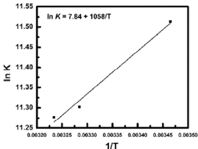
Fig. 4. Van't Hoff plot for Hb-SMZ binding from fluorescence quenching at 10 mM citrate phosphate buffer.
