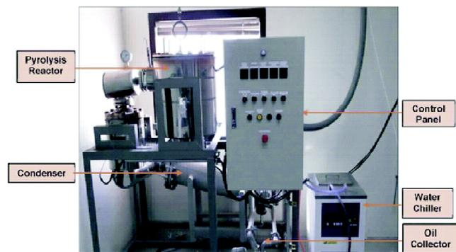
Fig. 2. Batch type pyro-reactor (Source: Miandad *et al.*<sup>44</sup>).
