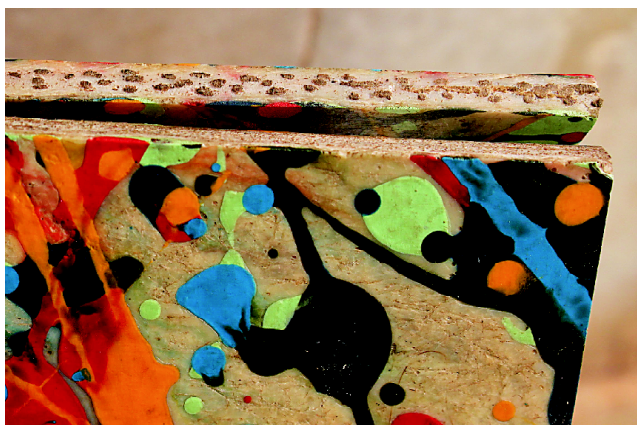
Fig. 11. Composite board from jute 2% NaOH scouring for 2 hours and mixed glue of ratio 70:30.
