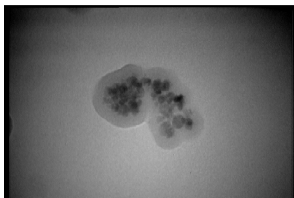
Fig. 3. TEM image of \gamma\text{-Fe}_2\text{O}_3\text{@CuO} nanocomposite.
