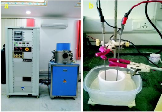
**Fig. 1.** Optical pictures of (a) RF/DC magnetron sputtering system and (b) electrochemical anodization.
