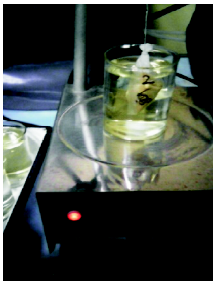
Fig. 1. Experimental setup of bio-adsorbent pack in dip-tea-bag for lead ion removal.
