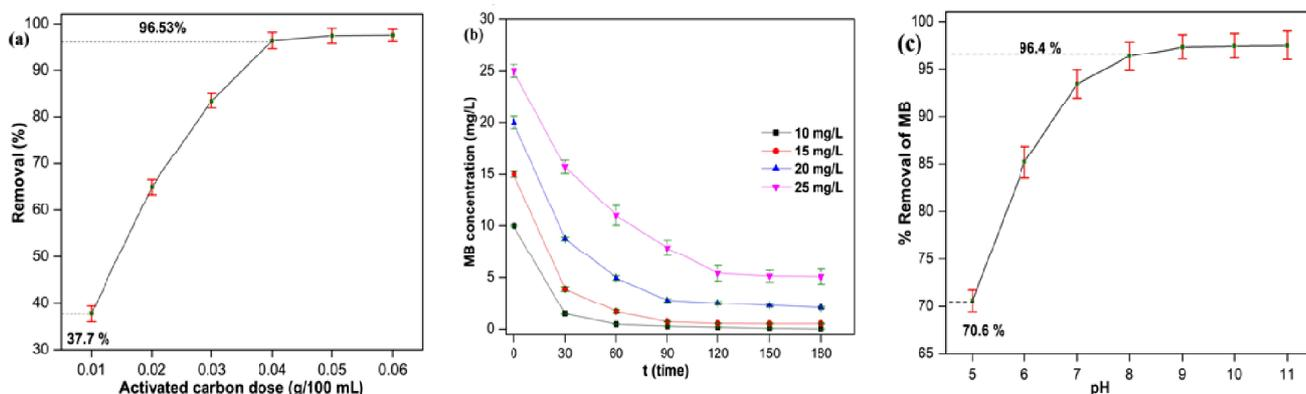
Fig. 2. (a) Effect of MSAC dosage on removal of MB (contact time ( $t$ ) = 180 min,  $C_0$  = 10 mg/L, temperature = 30°C, pH = 8.0). (b) Effect of contact time and initial concentration on MB adsorption (contact time ( $t$ ) = 180 min, adsorbent dose = 0.04 g, temperature = 30°C, pH = 8.0). (c) Effect of pH on MB removal ( $C_0$  = 10 mg/L, adsorbent dose = 0.04 g, contact time ( $t$ ) = 180 min, temperature = 30°C).
