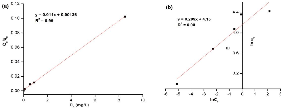
**Fig. 3.** (a) Linearized Langmuir isotherm for MB adsorption by MSAC, (b) linearized Freundlich isotherm for methylene MB adsorption by MSAC.
