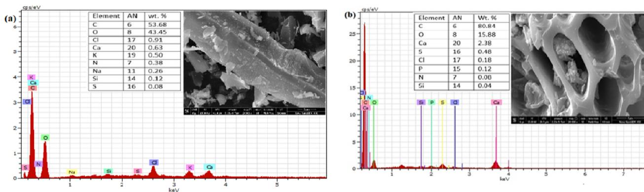
Fig. 1. FESEM image of: (a) MS and (b) MSAC prepared with  $ZnCl_2$  activation.
