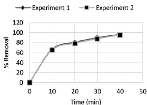
Fig. 6. Fluoride removal (%) vs time for tap water.
