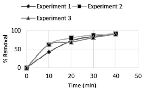
Fig. 4. Fluoride removal (%) vs time for voltage variation.
