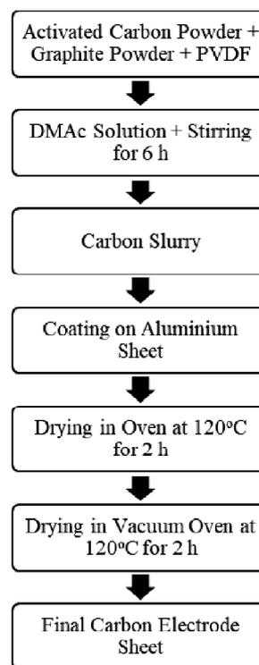
Fig. 1. Flowchart for steps involved in the carbon electrode sheet fabrication.
