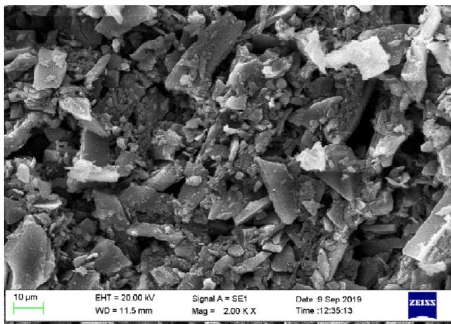
Fig. 3. SEM image of electrode after desalination process.
