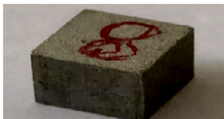
Fig. 2. Machined specimen (Exp. 8) (size: 6 mm×5 mm×5 mm).
