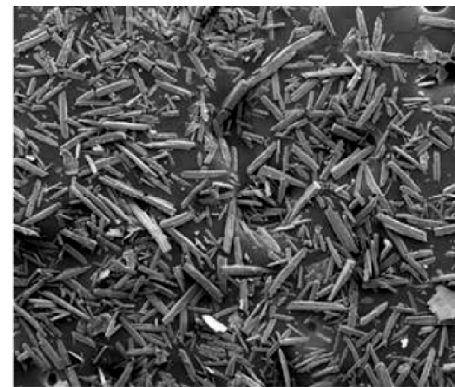
Fig. 3. Irregular crystals of struvite 28 .
