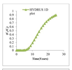
HYDRUS 1D predicted Chromium BTC through 1m vertical soil column to be used as liner material in waste containment structures.
