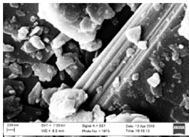
Fig. 4. SEM image of the \text{TiS}_2 as-received.
