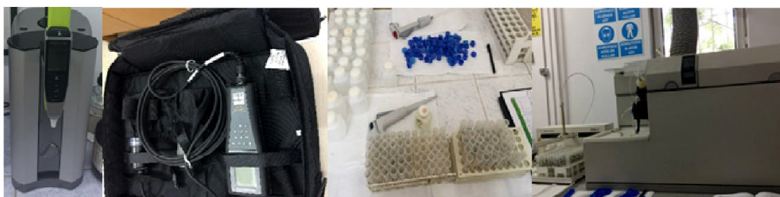
Fig. 1. (a) Elga Purelab Flex Deionized water, (b) YSI Professional plus multiparameter meter, (c) Sampling bottles and vials, (d) Autosampler (CETAC ASX-51) and ICP-MS (Agilent 7500a).
